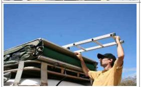
Slide out the ladder until the locking pins engage.
