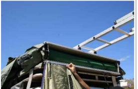
Feed the back wall of the Annex into the sail track that was occupied by the travel cover.
