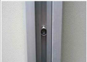
Slide 2 x 8mm nuts into each of the mounting rails and align them with the pre-drilled holes. Place the mounting extrusion into position over the bolts.
